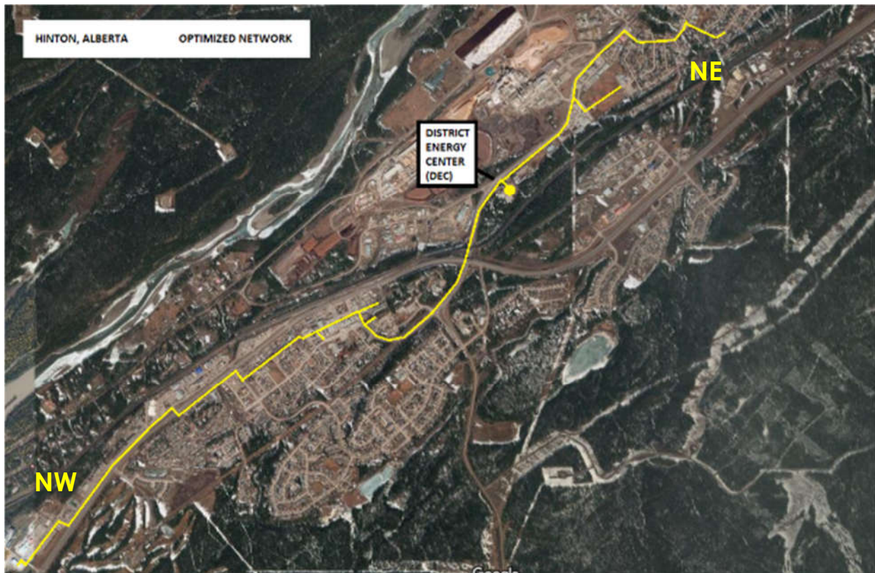
Figure 32 – Optimized Hinton DES, Proposed Distribution Network (38 Consumers, ZONES 1 and 2)
