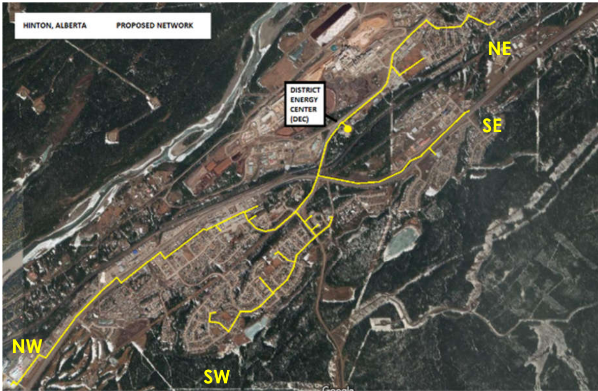
Figure 1 – Complete Hinton District Energy System, Proposed Distribution Network (53 Consumers, ZONES 1 to 4)
