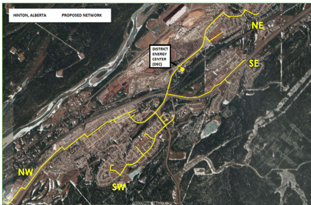
Figure 26 – “Complete” Hinton DES, Initial Proposed Distribution Network (53 Consumers)
